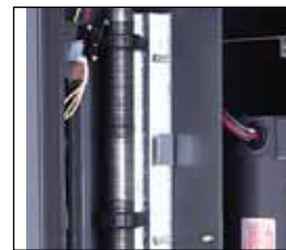
limit switches direct driven and easily adjustable
