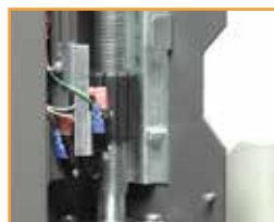
direct drive limit switches
